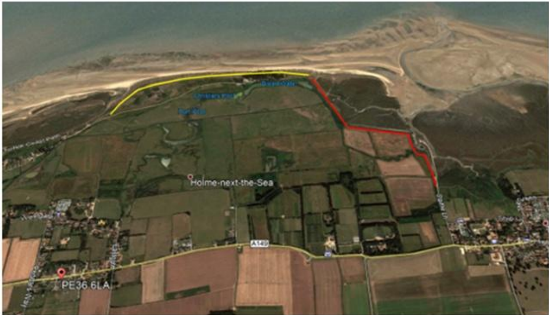
Figure 5: Thornham Sea Bank (red line) was built by the Le Strange Estate to enable reclamation of a much larger area in 1860. Protection to the north was provided by a timber and clay bank which provided the foundation for development of today's line of sand dunes which had formed by 1900.
